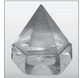
This glass prism with a slightly green tint is 4 1/2 inches high and very heavy. It was used like a window on vintage sailing ships to get light below the main deck. Just an ornament today, it is worth about $50 in an online sale.
